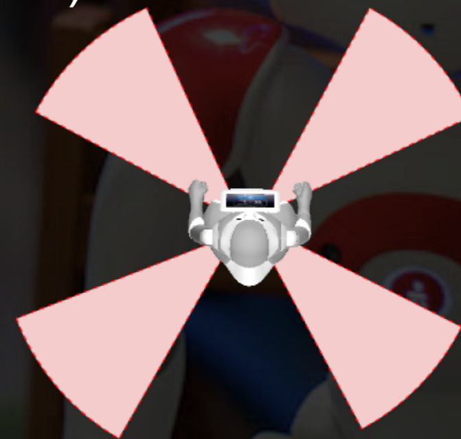
Pepper blind spots. Arm speed is reduced when moving inside these zones
