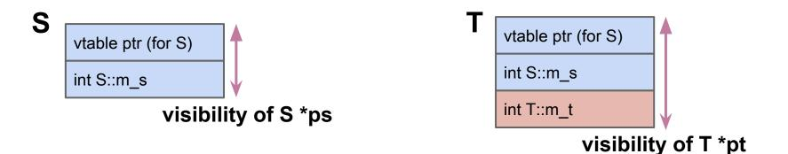
Memory region for T::m\_t can be corrupted using T\* pt as it was never allocated.
